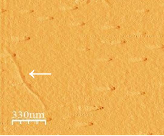
$\checkmark$  About 1 nanotube per  $\mu$ m: Nanotubes are correctly individualized.
